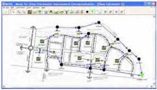
Using MUSIC, you can make a first estimate on the expected pollutant load from catchments following development, in the absence of any stormwater treatment initiatives. This sets a baseline condition which can then be used to compare alternative stormwater treatment strategies for compliance with state and local government stormwater quality objectives.
