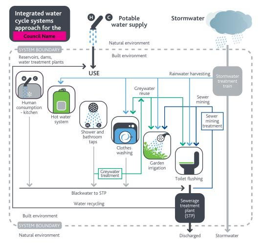
Figure 12. Integrated water cycle systems approach
