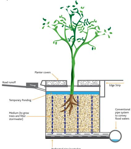
Perforated pipe located to drain filtered stormwater
