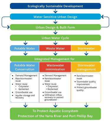
Figure 4. Interactions between ESD, WSUD and the Urban Water Cycle shows the close relationship between WSUD elements. Often links between the urban water streams are developed when one element is adopted, for example rainwater harvesting will conserve potable mains water and reduce stormwater discharges.
