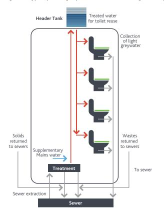
Water mining systems need a dedicated dual supply pipe to deliver the reclaimed water to toilets, cold washing machine tap and/or irrigation. Adequate provision of the pipe network is essential during the building's construction. Treatment technologies can be located in the basement of the building through 'package plants'.
