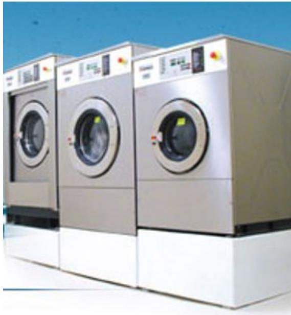
Pictured above right, Ipso 23, 16, and 9.5 kg washer extractors with WaterSaver® recycling tanks. Relatively inexpensive water recycling tanks doubling as a plinth to raise loading height of washers. Compatible with Ozone Laundry technology these tanks are proving to be quite popular in aged care facilities across Victoria. Expected water savings of 20% are achievable with this type of system.
